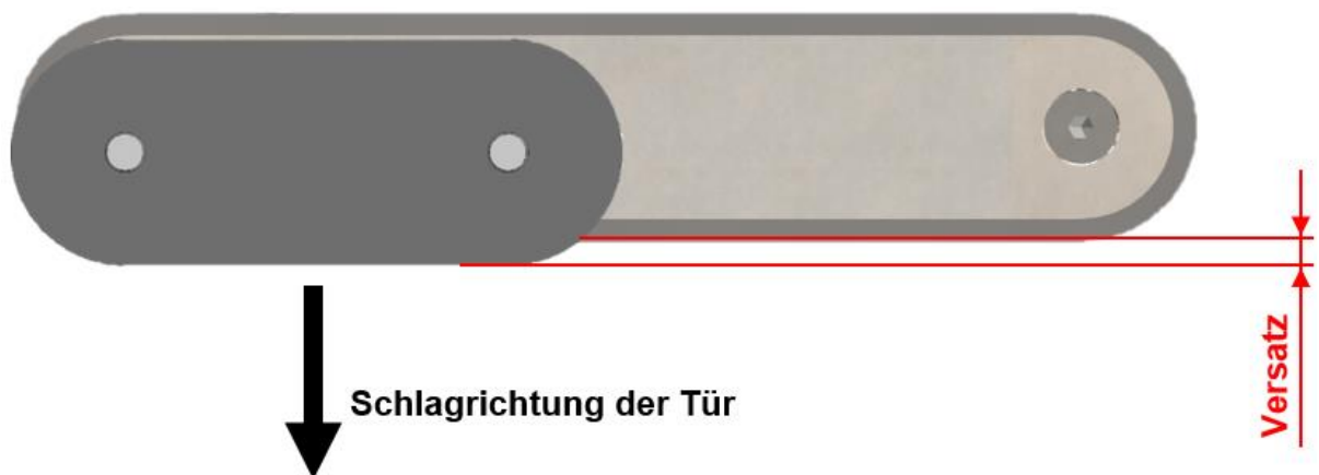
Figure 2 : Coinciding distance between locking device and striking plate
